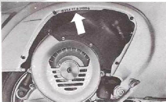
Fig. 24 - Serial number stamped on frame.
